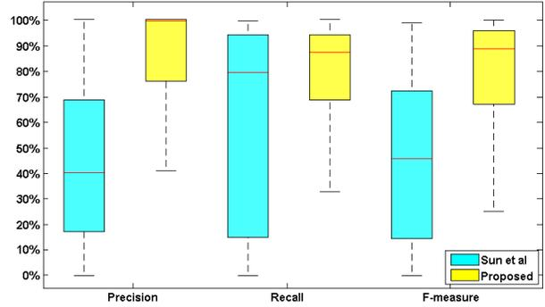
**Figure 5: Comparison with Existing Technique****Table 2: Comparison with an Existing Technique**
